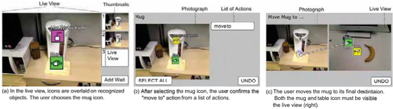
Fig. 2. Creating an instruction to move a mug from a hot water kettle to a table.
