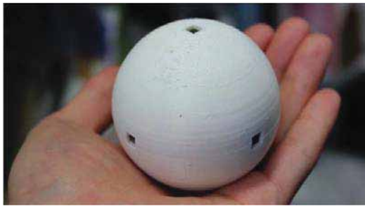
Figure 10: Photograph of FuwaFuwa sensor module (3 of the 6 photoreflectors are visible)
