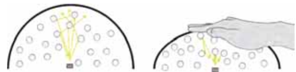
Figure 2: Directionality of reflected light is lower at low density (left) than at high density (right).
