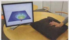
The FuwaFuwa technology gets even more interesting when you consider that multiple sensor modules can easily be tucked away inside a pillow or cushion. By correlating the data from several sensors the object can become a video game controller, a musical instrument keyboard, a robot that responds to touch or caresses on different parts of its body, or a wide range of other useful things.
