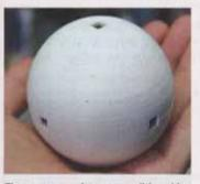
The raw sensor data, preconditioned by the onboard microprocessor, can be easily analyzed remotely to determine the relative pressure location in a 2D plane and the relative magnitude of the applied pressure. I suspect that for most practical applications relative measurements will be more than satisfactory rather than absolute, closely calibrated measurements.
