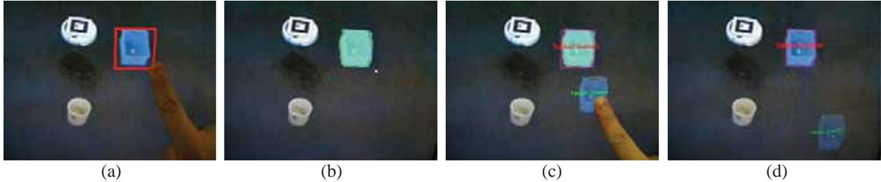
Fig. 1. Drag-and-Drop Operation by the User—(a) The user selects the target object. (b) The system highlights the selected object. (c) The user drags the object. (d) The user drops it at the target location. The robot then autonomously pushes the target object to the target location.
