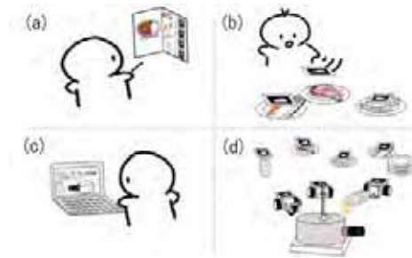
Figure 4: Scenario with recipe book. (a) User chooses recipe, (b) preprocesses ingredients and places markers, (c) starts system, and (d) system begins cooking.
