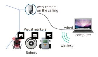
Figure 2 Example setup of the toolkit
