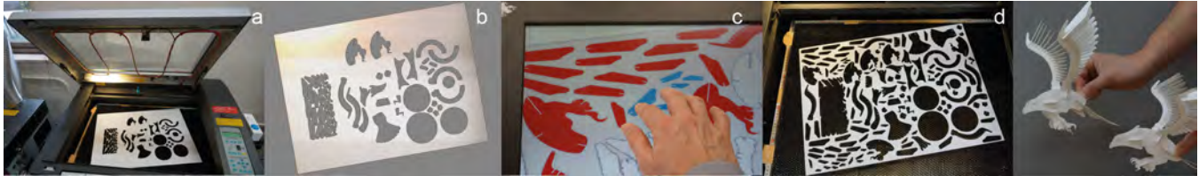
Figure 1. PacCAM supports users in packing 2D parts by capturing materials in a CNC machine (a) and using the captured materials (b) in a dedicated user interface based on 2D rigid body simulation and snapping (c), resulting in optimized utilization of material for efficient fabrication (d).
