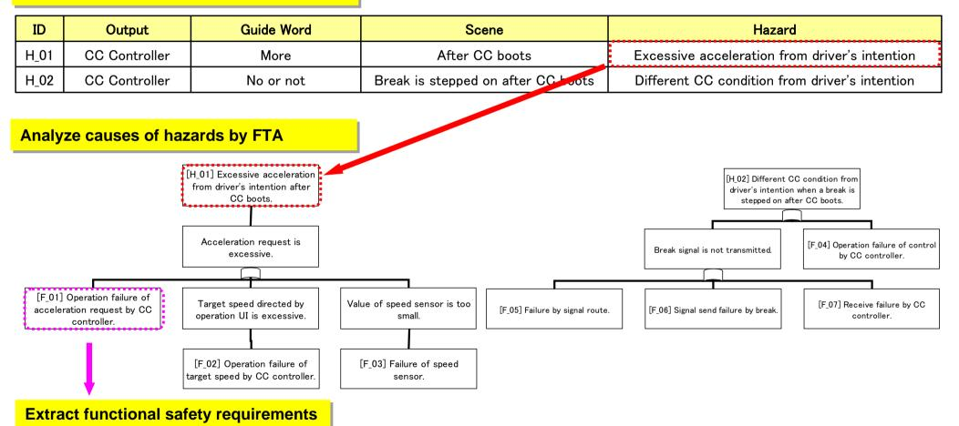
Control which keeps acceleration in tolerance level can be performed even when an operation failure occurs by CC controller.
