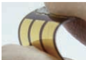
High-efficiency perovskite solar cell fabricated on plastic film.
