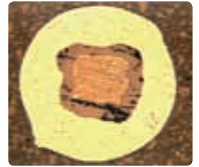
Cross sectional photograph (prior to heat treatment) Diameter: 0.88 mm
