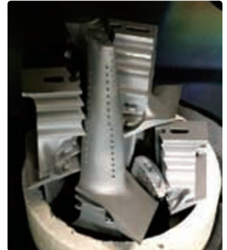
We conduct research on recyclable technology that re-uses a turbine blade as a material having the equivalent or more of the original superalloy by re-solving the used nickel-base superalloy turbine blade in calcia crucible, removing impurities such as sulfur.
