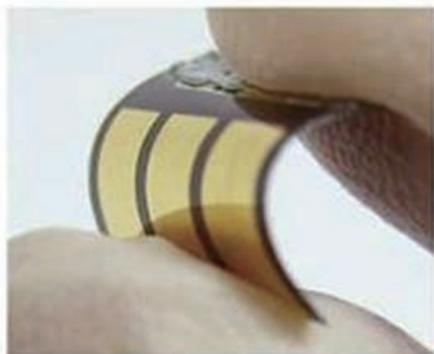
High efficiency perovskite solar cells made on plastic film. They retain stable performance levels even after being put through experiments in which they are bent 100 times or more.
