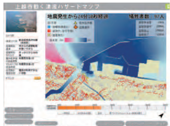
One example of 'dynamic hazard maps'
