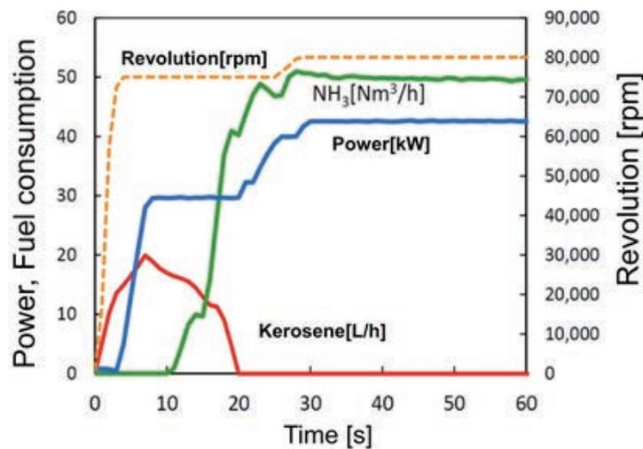
NH<sub>3</sub>/air fueled operation (Power generation: 41.8 kW)
