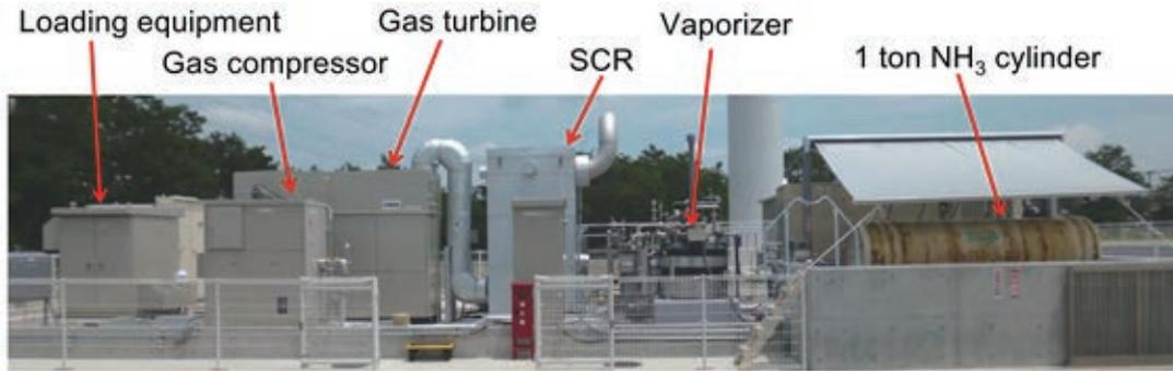
NH<sub>3</sub> gas-turbine test facility in AIST
