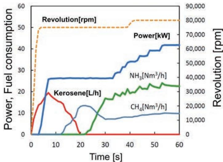
NH<sub>3</sub>/CH<sub>4</sub>/air fueled operation (Power generation: 41.8 kW)
