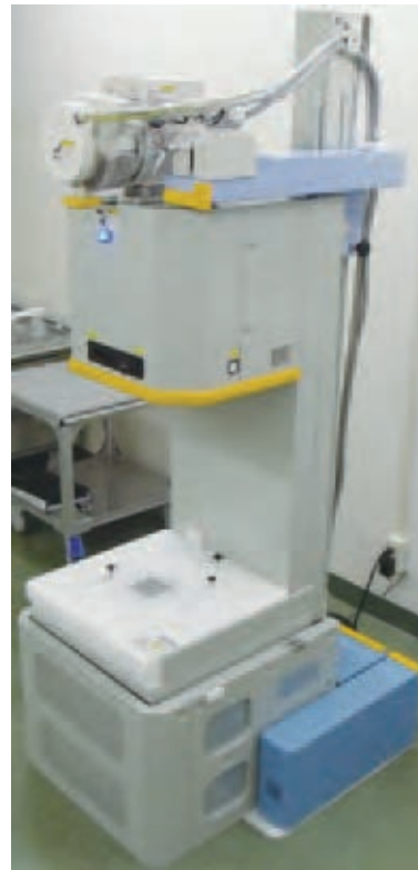
Prototype X-ray photography apparatus (vertical model) (Provided by, Konica Minolta Inc.)
